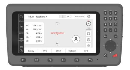
According to the actual needs of front-line surveyors, the Alpha Android total station panel is designed with a 5.5-inch touch screen + physical buttons, which takes advantage of the operating advantages of the Android system and is more in line with measurement habits. Outstanding hardware and professional software make measurements easy.
